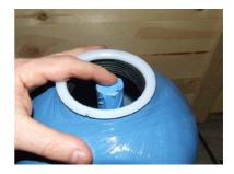
Once the riser tube is centrally positioned into the empty vessel, start to fill the vessel with mixed bed resin. A cut down funnel is a useful tool to assist filling. Fill the vessel up to the shoulder position, as indicated. Shake the container frequently to ensure a good settlement and compaction of resin. Do not overfill and ensure that the riser tube remains central during the procedure.
