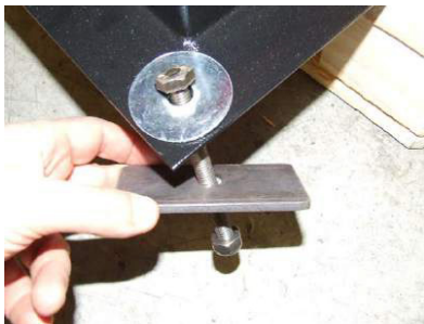
Always ensure that the metal plate is placed on the underneath of the vehicle against the floor plan or chassis member. Position round washer with the bolt on the inside of the van.
