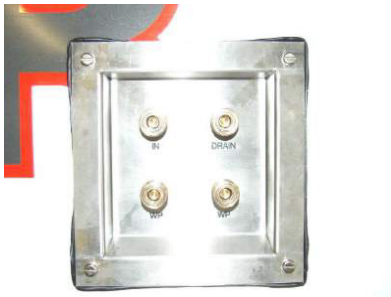
This is how the front of the manifold should look from the outside of the van.
