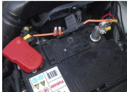
Here is an example of how to wire up the vehicle battery. There is a fuse holder on the red - positive. This is how you will receive the wiring loom.
