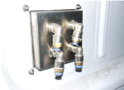
This is an example of how the manifold should look from the inside of the van.
